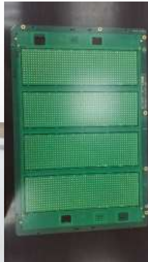
4 layer PCB, inner layers printed
